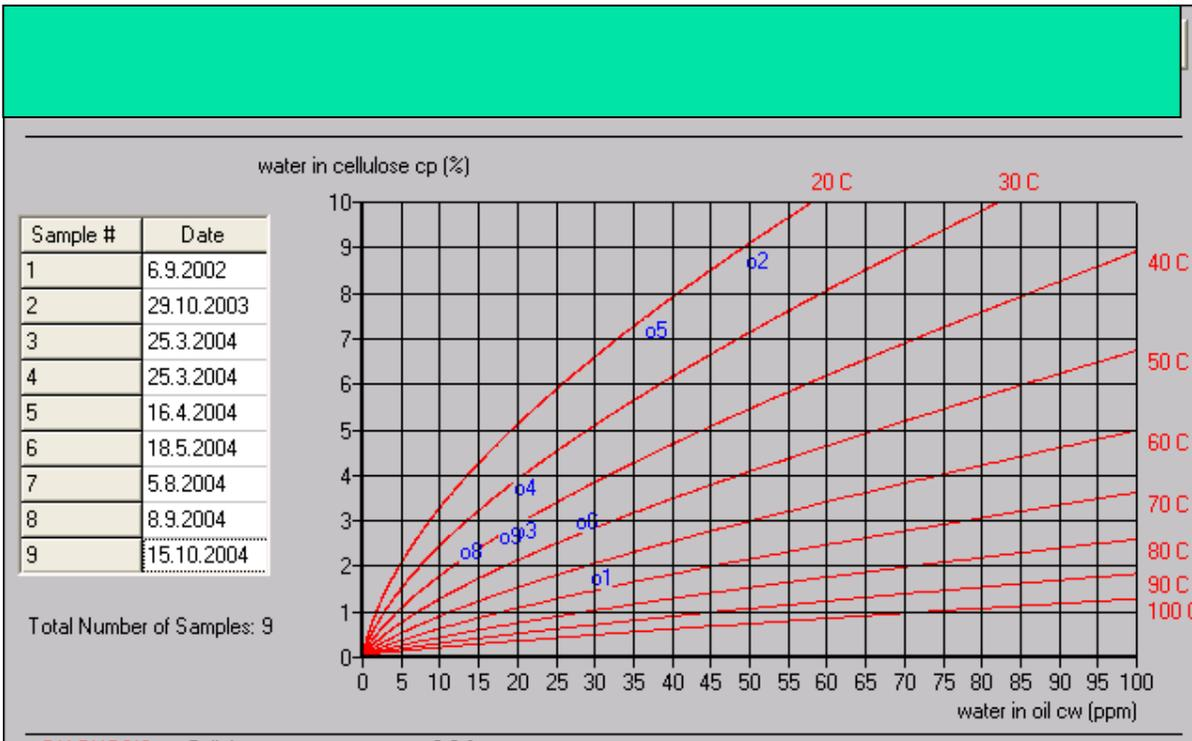
Measurements 6 and 9 were based on the relative moisture, whereas value 9 reflects a certain drying effect achieved with the bypass system. An FDS measurement conducted at time 6 yielded a result of 3.1%. The water separation achieved with the bypass system points to a similar value. The other values were achieved by conventional measurements whose fluctuation range alone makes them useless.
