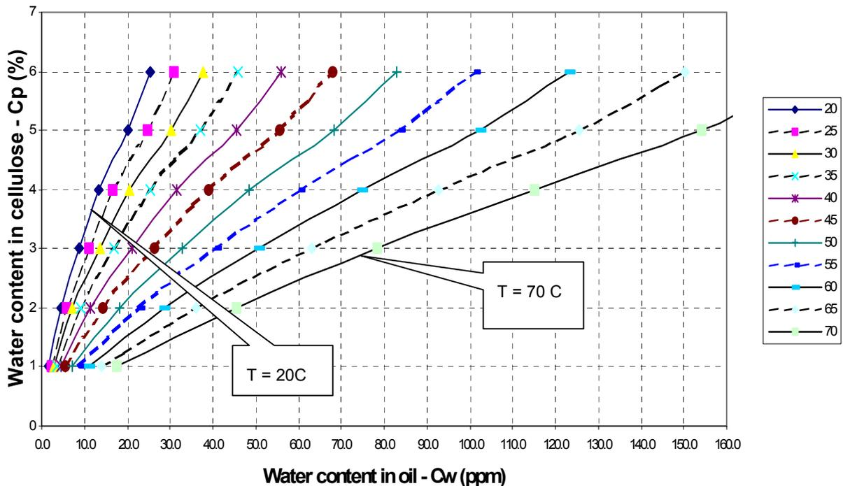
Fig.7 Nielsen diagram based on experiment data, (new oil NN = 0.005)
