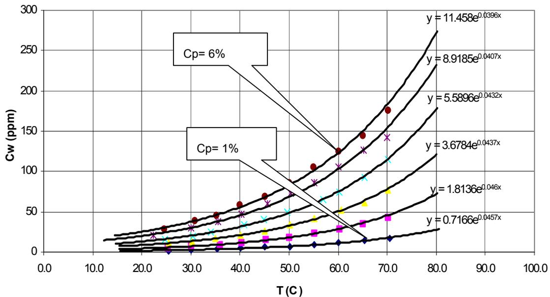
**Fig. 2** Relation  $C_{w,KF} = C_{w,KF}(C_p, T)$ ,  $NN < 0.005$  mg KOH/g, KF method
