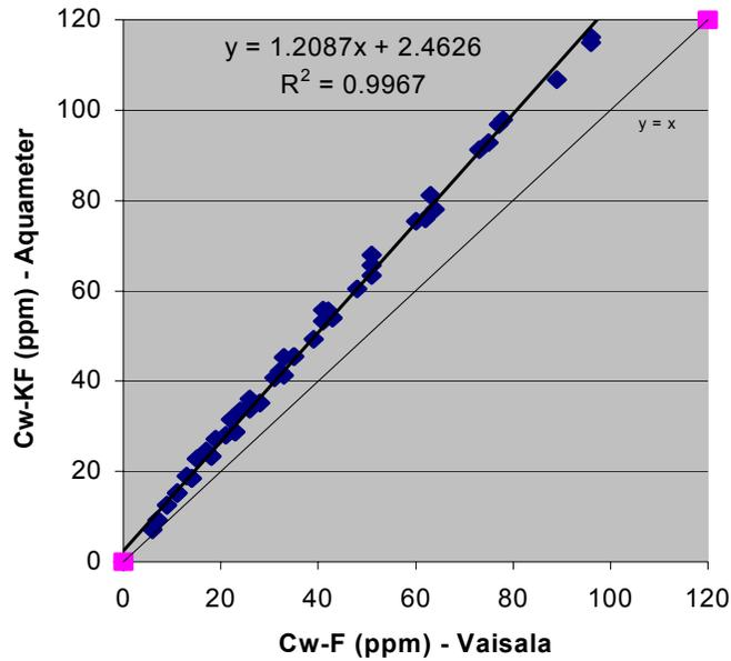
**Fig. 5** Aged Oil (NN = 0.18 mg KOH/g) - Correlation between the KF and F method -
