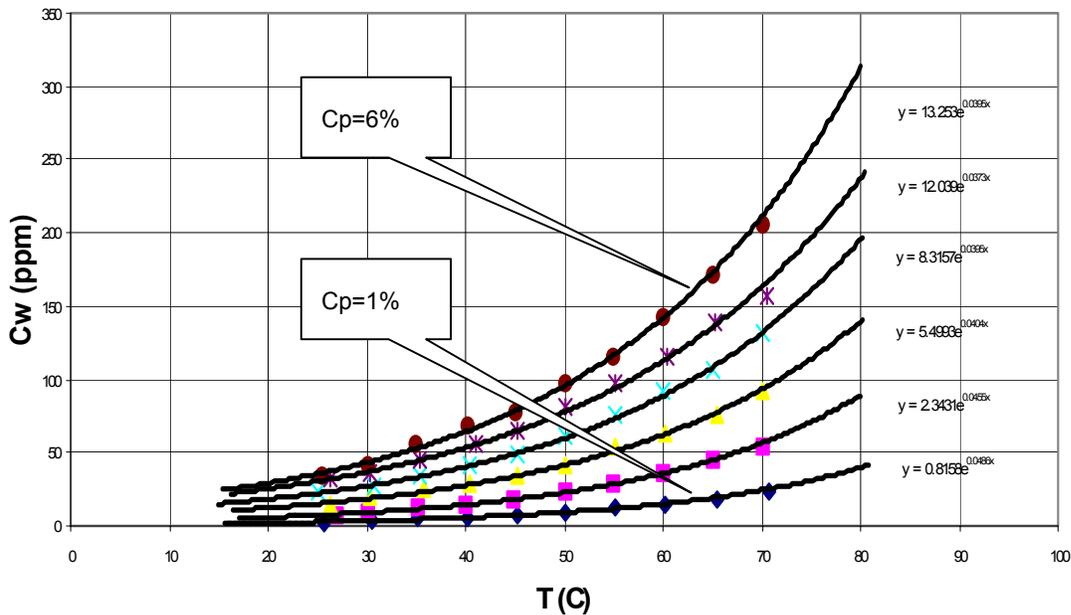
**Fig. 4** Aged Oil ( $NN = 0.18 \text{ mg KOH/g}$ ) - Relation  $C_w = C_w (C_p, T)$ , KF Aquameter method.
