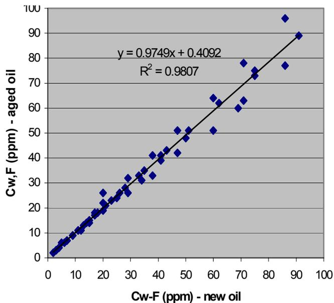
**Fig. 6** Correlation of sensor F methods: new oil versus aged oil (NN = 0.18 mgKOH/g)
