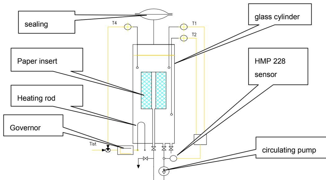
**Fig.1** Oil-cellulose moisture equilibrium simulator
