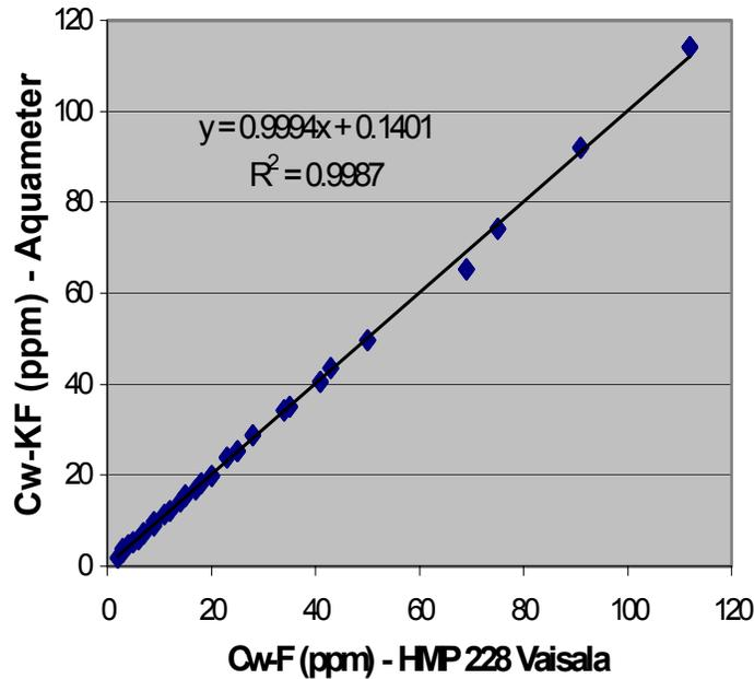
**Fig. 3** New Oil - The correlation of KF versus Sensor F method.
