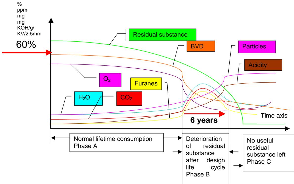
The following diagram is based on the presumption of typical populations with a homogeneous procurement age:
