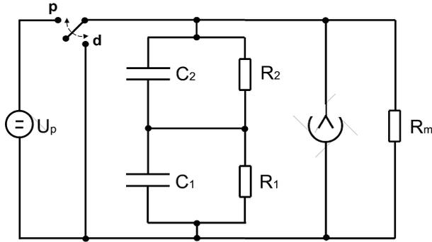
**Fig. 2:** Equivalent circuit of a paper-oil-dielectric with  $\tau_2 = R_2 C_2$  and  $\tau_1 = R_1 C_1$  and basic measuring circuit
